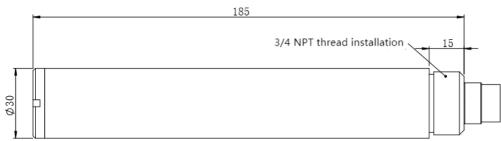
Note: The sensor joint is M16-5 core waterproof joint male head
