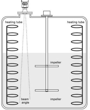
The extremely low launch angle ensures accurate measurements even under extremely harsh conditions.
